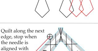
Use the reference lines to make a narrower wedge design. Quilt along the first side as normal, repositioning the ruler when you get to the point.
